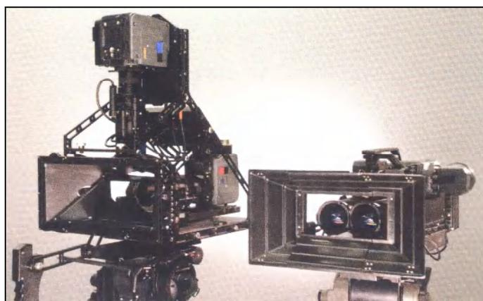
図 2.1-17 Fusion 3-D Camera System
